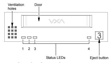
Figure 1-2 Internal tape drive: front-panel components
